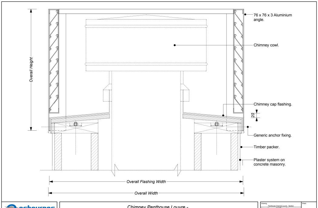
OSBOURNES diffusers grilles and louvres <u>Chimney Penthouse Louvre -</u> <u>Typical Section</u>
